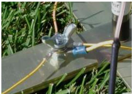
7) Place the lug from each of the three radial wires over the ground lug and secure them tightly with the wing nut. Arrange the Radial Wires in an equally-spaced triangular pattern from the base.
