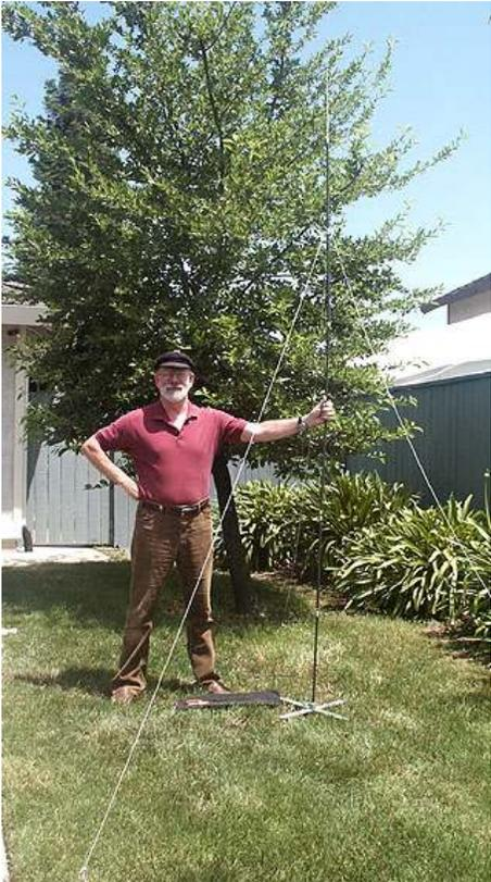
The HFp antenna, assembled in its 40 Meter configuration, with included guy lines attached. It's about 11 feet tall – you can just see the top whip against the tree background. If the guy lines were black, it would almost completely disappear!
