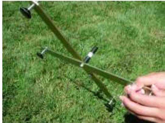
2) Insert the base insulator bolt with its split lock washer through the holes in **both** pieces of aluminum and install the Base Insulator on the bolt. Tighten the insulator, while holding the two base plates to form them into an "X", as shown.
