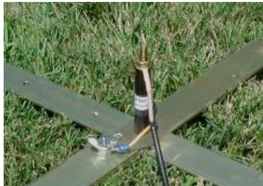
5) Place the center conductor lug of the coaxial pigtail over the top hole of the Base Insulator and use an Inter-Element Connector (IEC) to hold the lug in place.
