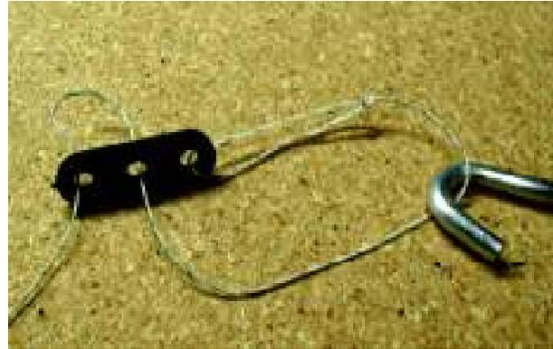
The slider moves very easily toward the antenna, tensioning the guy line. To loosen the slider, grasp and hold the guy line on the antenna side of the slider, turn the slider slightly with your other hand, and slide it toward the stake.
