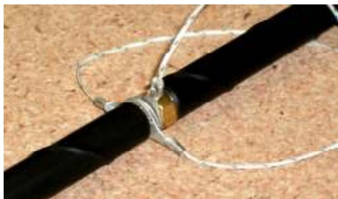
At the other end of the Guy Line, the line is threaded through two of the holes in the Guy Line Slider, and is tied to the third hole. A bowline knot is recommended here.
