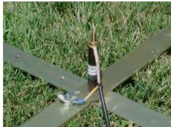
6) Put the coax shield lug (the black wire) on the ground stud, then screw the wing nut on top of it - not tight - you will need to take it off in a minute. Then place the base on the ground or another flat surface.
