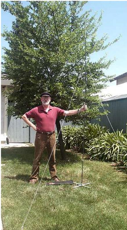
The HFp antenna, assembled in its 40 Meter configuration, with included guy lines attached. It's about 9 feet tall – you can just see the top whip against the tree background. If the guy lines were black, it would almost completely disappear!
