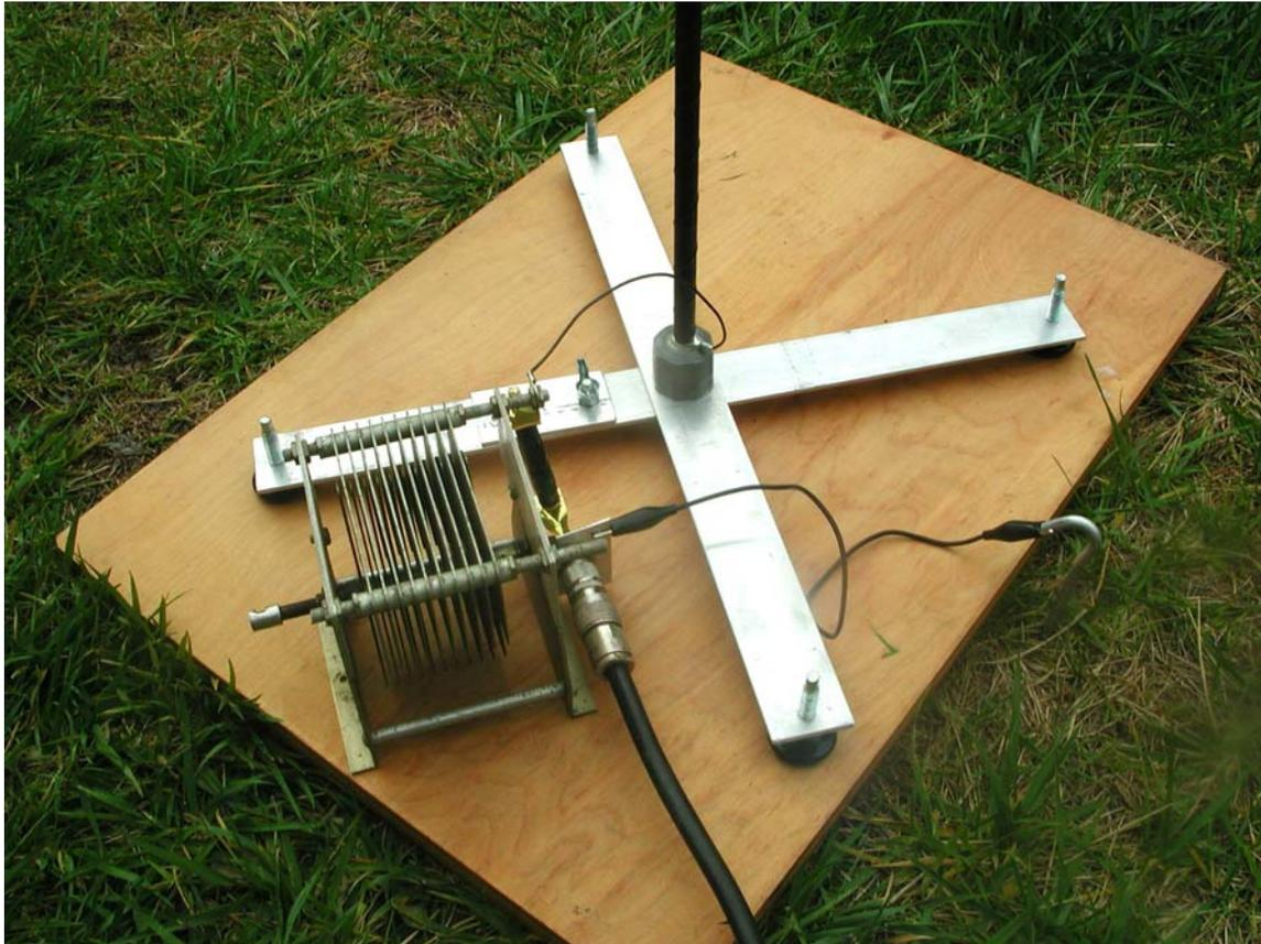
The coil (L) is the little tubular vertical thing at the end of the coax connector. It connects to the top of the capacitor, and then by a small wire to the base of the antenna. You can see the guy stake, and the clip lead connecting the outside of the coax and one side of the capacitor to ground. I set the antenna base on a piece of wood so that the grass wouldn't get into the capacitor plates.
