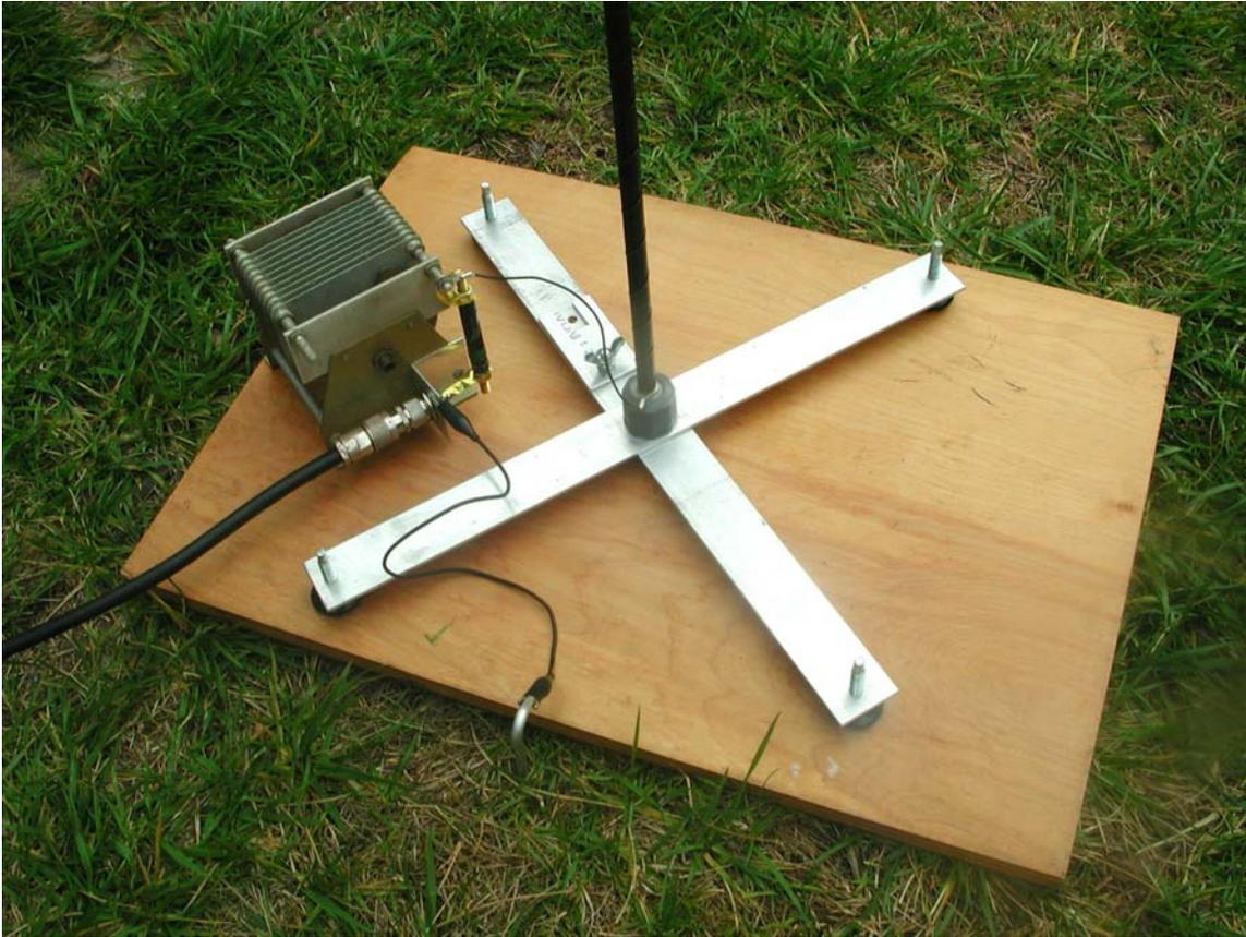
When adjusting the antenna and the matcher, you will find that there is a bit of interaction between the two units, and it will take a couple of adjustments if you want to get the SWR down to its lowest at the target frequency. This means taking the antenna down, moving the whip in or out a bit to move the resonant frequency, re-installing the antenna, and then some radio or analyzer tests while adjusting the capacitor for best SWR.
